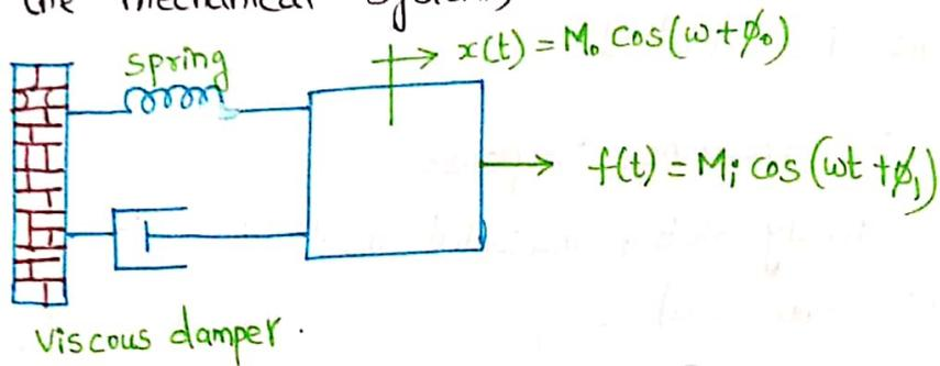
If the input force  $f(t)$  is sinusoidal, the steady-state output response  $x(t)$  of the system is also sinusoidal and at the same frequency as the input.
