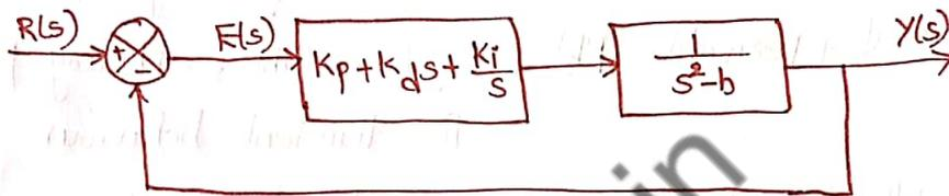
$$\frac{Y(s)}{R(s)} = \frac{K_p + K_d s + \frac{K_i}{s}}{s^2 - b} \cdot \frac{1}{1 + \frac{K_p + K_d s + \frac{K_i}{s}}{s^2 - b}}$$
