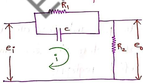
$$R_1 \parallel C \quad \text{then} \quad z = \frac{R_1}{Cs} + 1 + \frac{1}{Cs}$$
