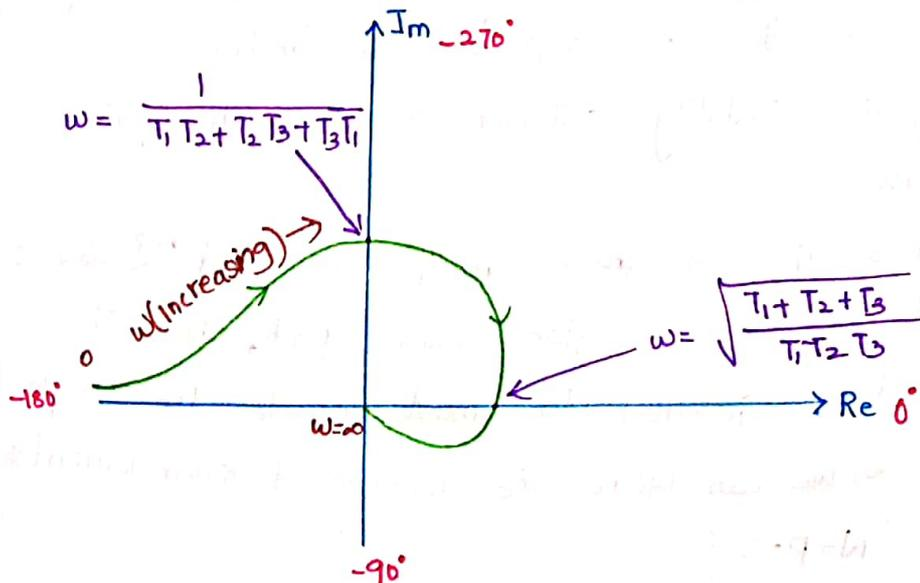
1) Addition of pole at origin to Transfer function rotates the polar plot by  $-90^\circ$  as  $\omega \rightarrow \infty$  for  $\forall \omega$  and
