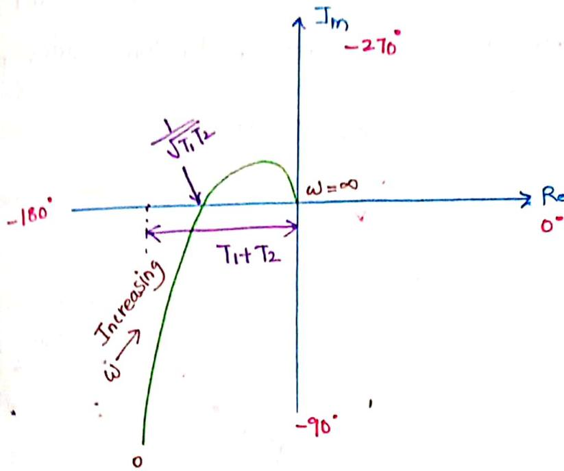
$$⑥ \quad G(s) = \frac{1}{(j\omega)^2(1+j\omega T_1)(1+j\omega T_2)}$$
