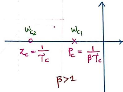
$$\frac{F_o(s)}{F_i(s)} = \frac{(R_2 + \frac{1}{Cs}) I(s)}{(R_1 + R_2 + \frac{1}{Cs}) I(s)}$$
