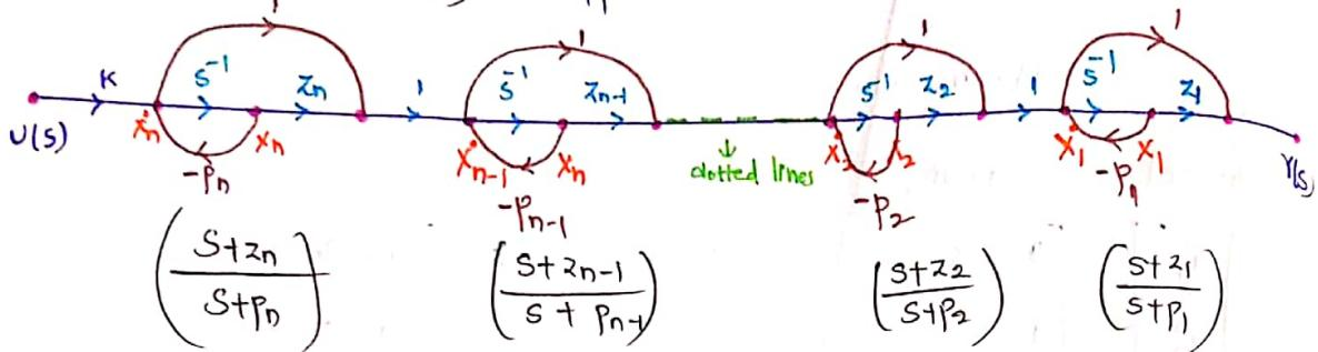
$$\left( \frac{s+z_n}{s+p_0} \right), \left( \frac{s+z_{n-1}}{s+p_{n-1}} \right), \left( \frac{s+z_2}{s+p_2} \right), \left( \frac{s+z_1}{s+p_1} \right)$$
