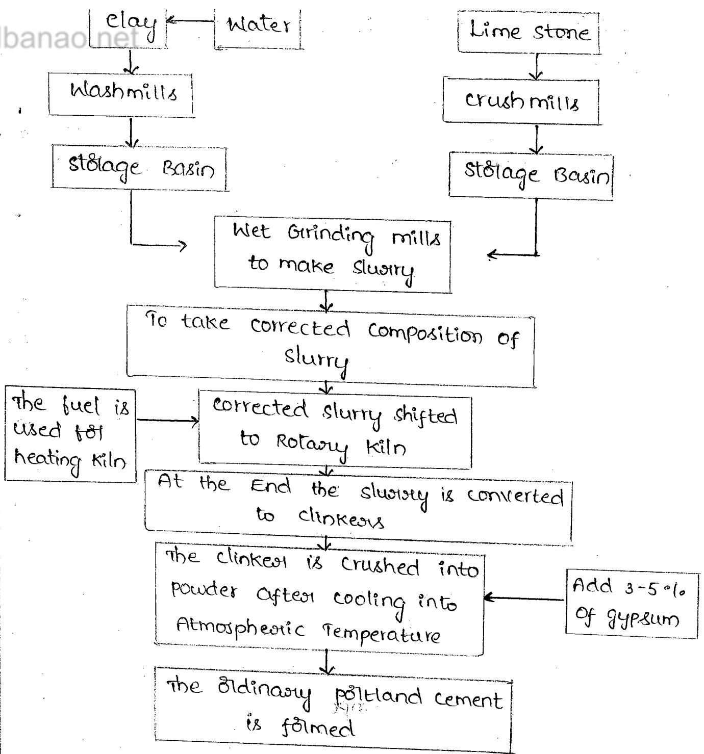
those are Lime, Alumina & silica in recombined state. After completion of oxidation reactions a hardened clinkers are deposited at the end of rotary kiln. the cooling process takes place in various conditions. After that the clinkers are powdered & adding 3-5% of Gypsum to form O.p.c.
