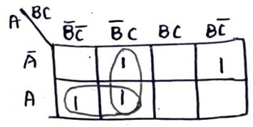
$Y = A\bar{B} + \bar{B}C + \bar{A}\bar{B}\bar{C}$
