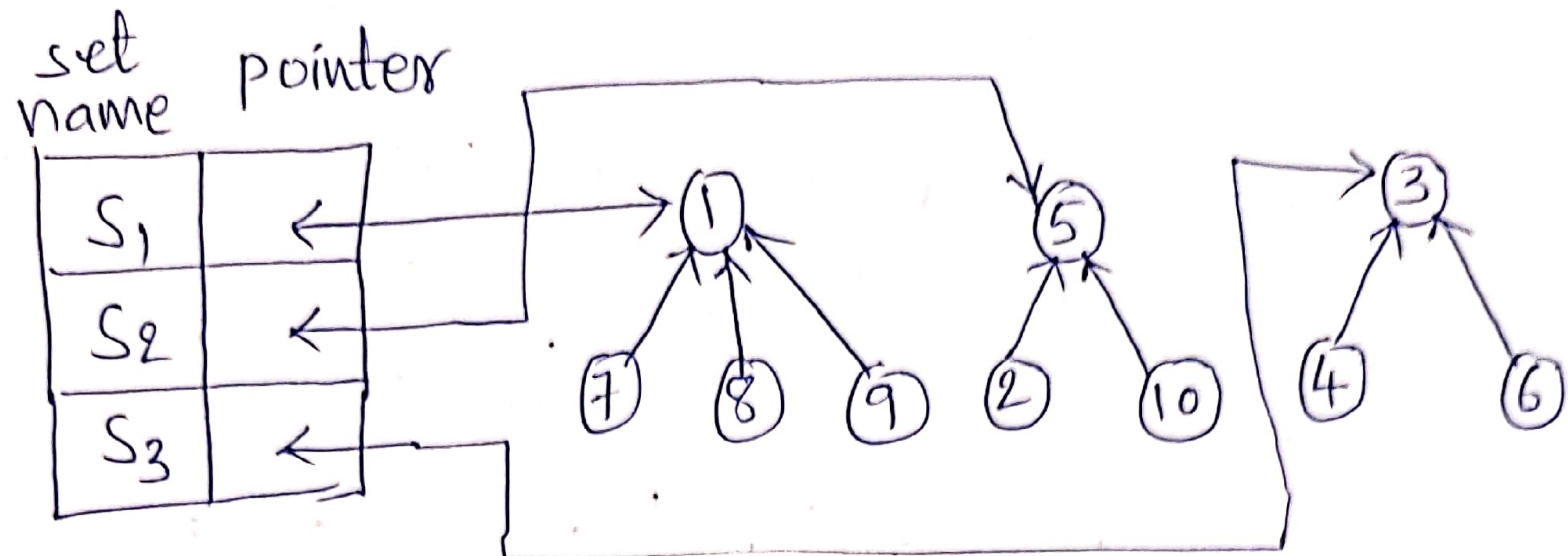
With each set name, we keep a pointer to the root of the tree representing that set. In addition, each root has a pointer to the set name. Then to determine which set an element is currently in, we follow parent links to the root of its tree.
