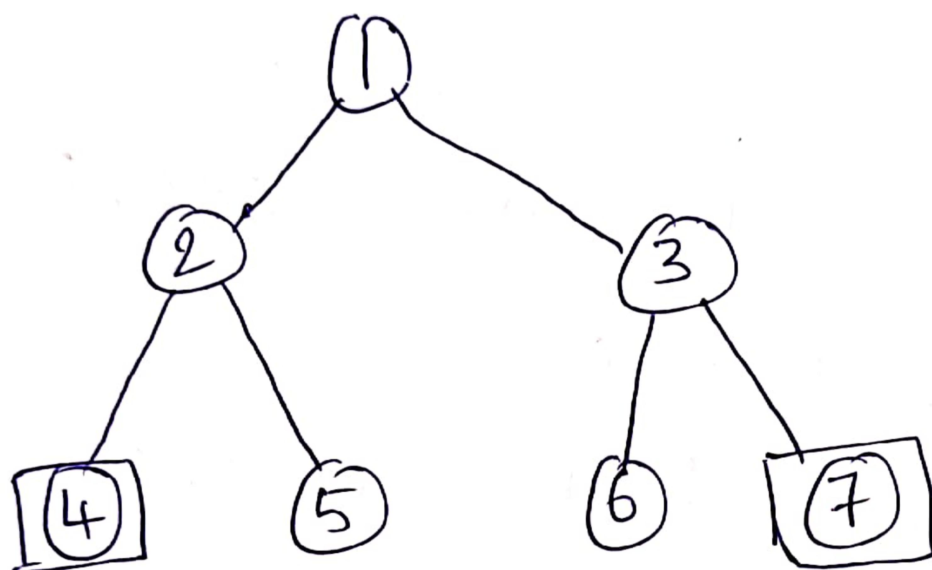
solution states are represented in the form of tuples. In above state space tree solution states are (1,2,4) and (1,3,7).
